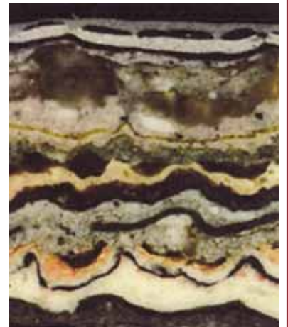
Microscopic view of paint layers © Naylor Conservation, 2008
